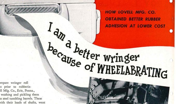
O prepare wringer roll shafts prior to rubberizing, Lovell Mfg. Co., Erie, Penna., had been washing and pickling them in stainless steel tumbling barrels. These barrels, with their loads of shafts, went through a cycle of alkali cleaning, rinsing, pickling in acid, etc. At best the job was performed under disagreeable working conditions because of fumes and dampness.
